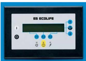
The versions Multi and Multi Dry are equipped with an electronic regulator "**ES ECOLIFE**". User-friendly, this device controls the operation of the various modules optimizing their use according to the compressed air request and levelling their respective operation hours.
